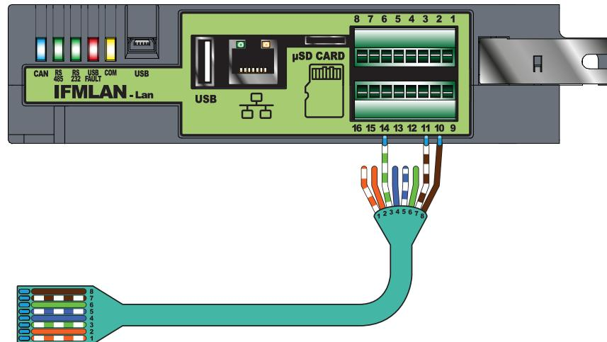
PREVIDIA-C-COM has two RS485 ports, both usable with a connection such as the following:
