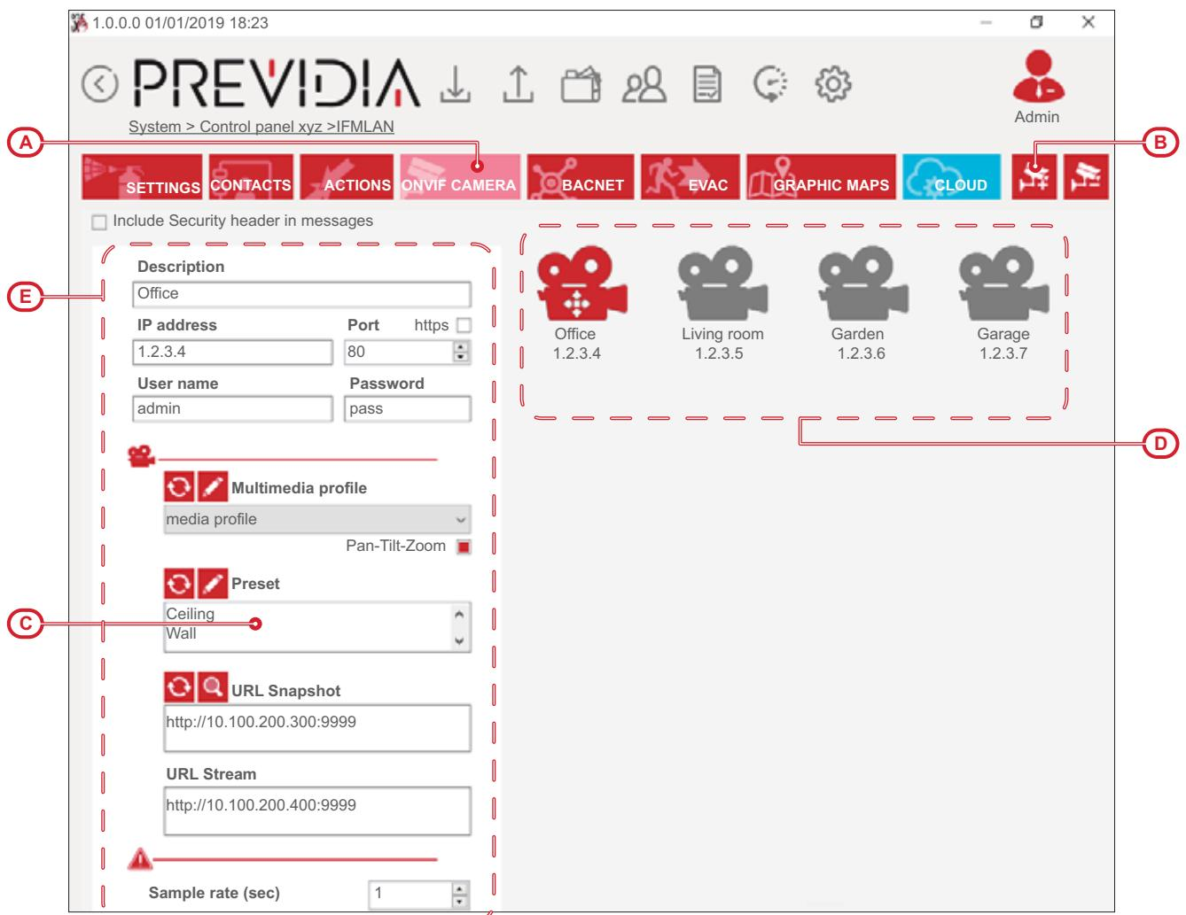
The section on the right [D] contains a list of all the configured IP cameras, while the section on the left [E] contains the parameters of the selected camera.
