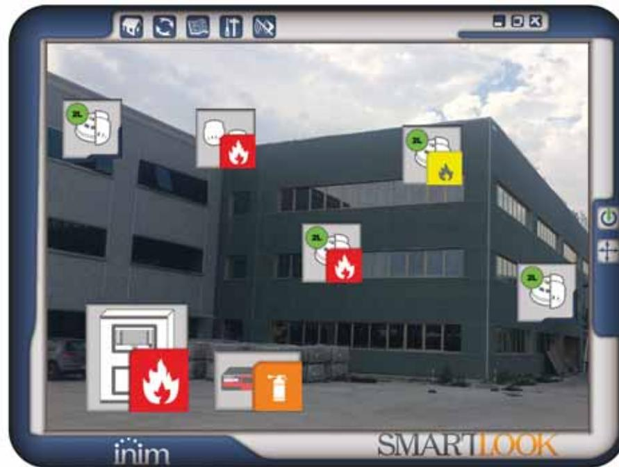
SmartLook uses Modbus over TCP/IP to communicate with the control panel (refer to paragraph 3.1 Modbus RTU and Modbus over TCP/IP). During the configuration phase, SmartLook asks for the addresses of Previdia control panels on the Modbus and Hornet+ networks.
